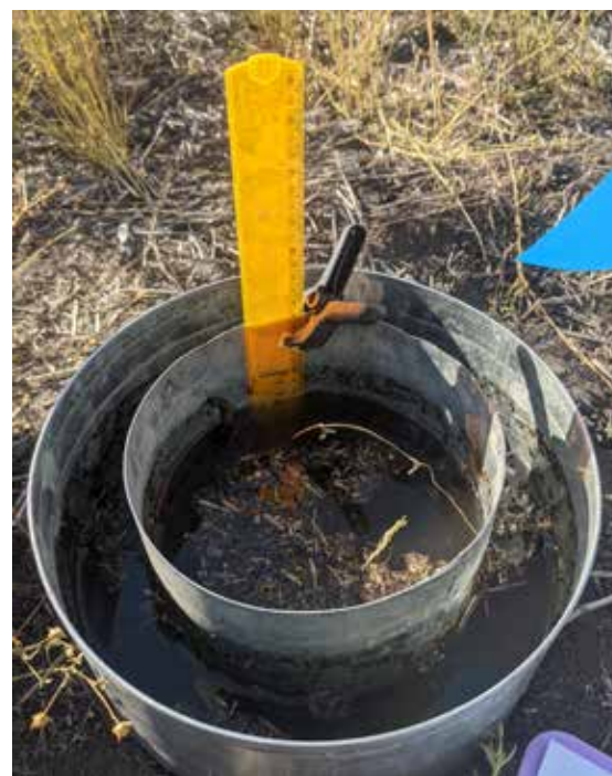
FIGURE 14. Double-ring infiltrometer used for water infiltration assessment.
